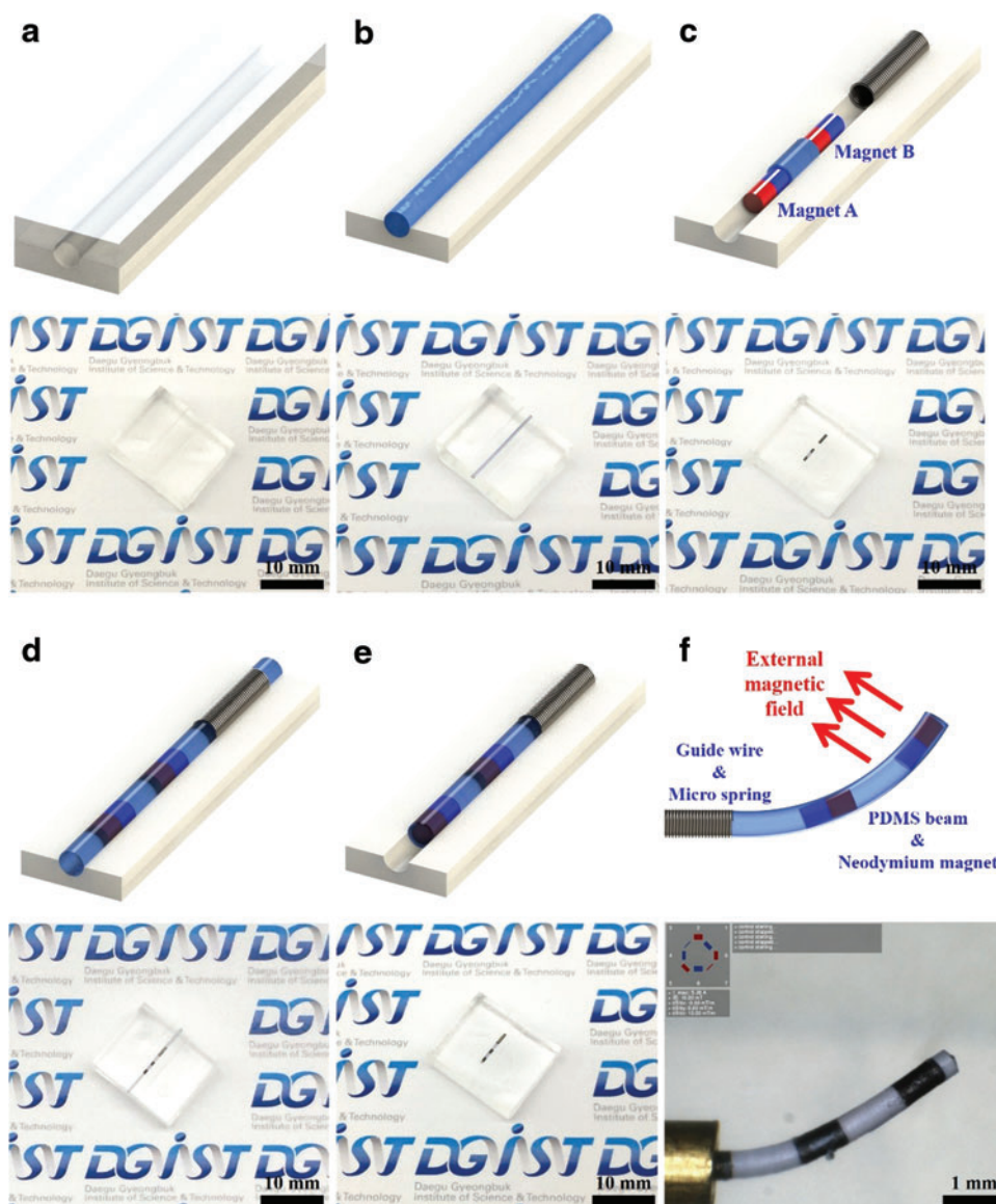
FIG. 5. Fabrication of the soft microrobot composed of a beam (polydimethylsiloxane [PDMS] silicone and a neodymium magnet), a connection (a microspring), and a guidewire. (a) The PDMS metal master mold and replica molding using PDMS; (b) pouring of the silicone elastomer mixture into the metal PDMS master mold, and curing; (c) alignment of the two-magnet, 1-mm-diameter rod-shaped PDMS block and the microspring; (d) pouring of the silicone elastomer mixture into the PDMS master mold, and curing; (e) adjusting the length of the microrobot; and (f) connecting the microrobot to the guidewire to allow guidewire steering. Color images are available online.
