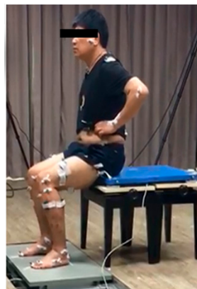
Figure 1. Sensors attached to a participant to detect eight bilateral Electromyography signals.
