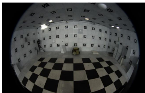
Figure 3. Fisheye camera image with distortion.
