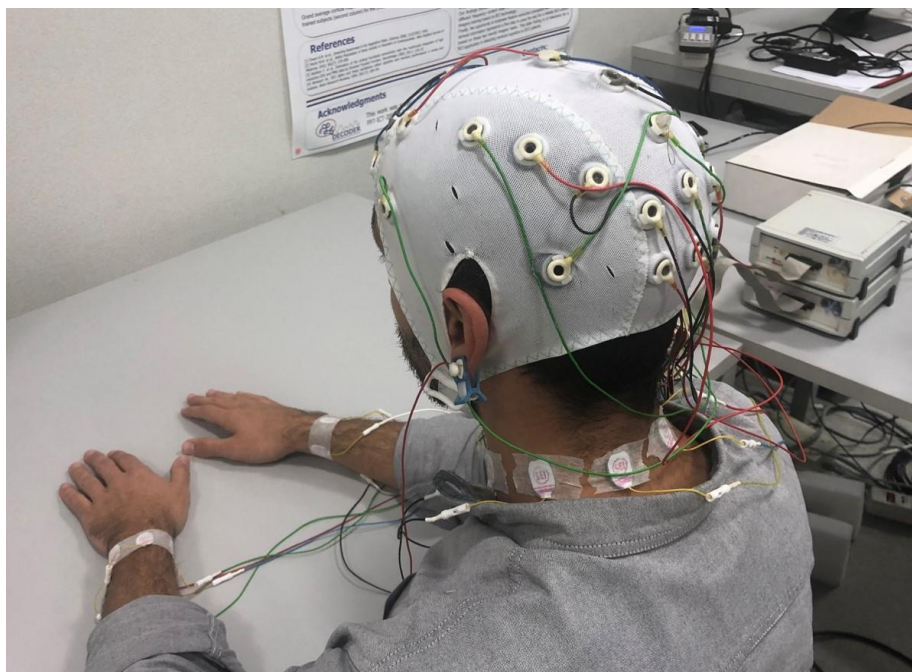
Figure 1. Participant wearing the electroencephalogram ( EEG ) cap and the noEEG sensors around the neck and wrists while seating comfortably and keeping the eyes closed.
