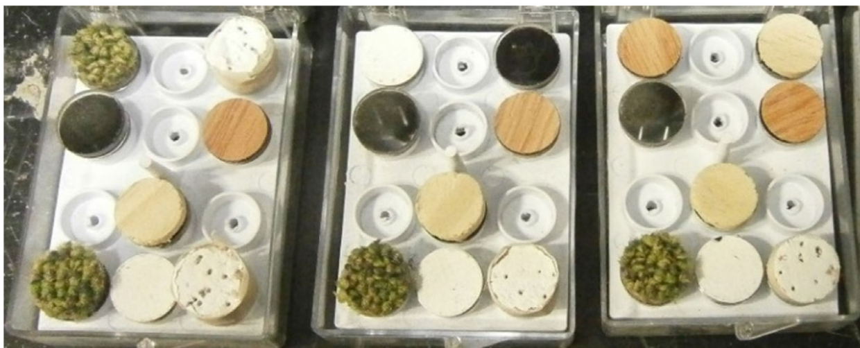
Figure 1. Photograph of 18 mm diameter coupons of materials mounted on stubs and placed in holder trays. [Colour figure can be viewed at wileyonlinelibrary.com ]
