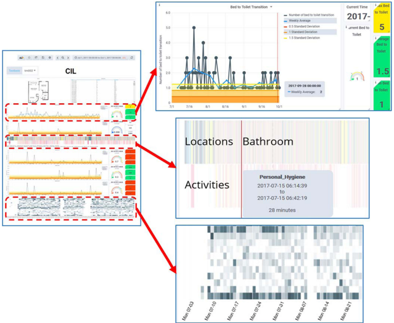
Fig. 4. (left) CIL interface. (upper right) Expanded view of line graph depicting daily number of bed-toilet transitions, together with rolling baseline. (middle right) Expanded view of time-aligned graph showing distribution of time spent among different activities and home locations. (lower right) Expanded view of activity level heat map.
