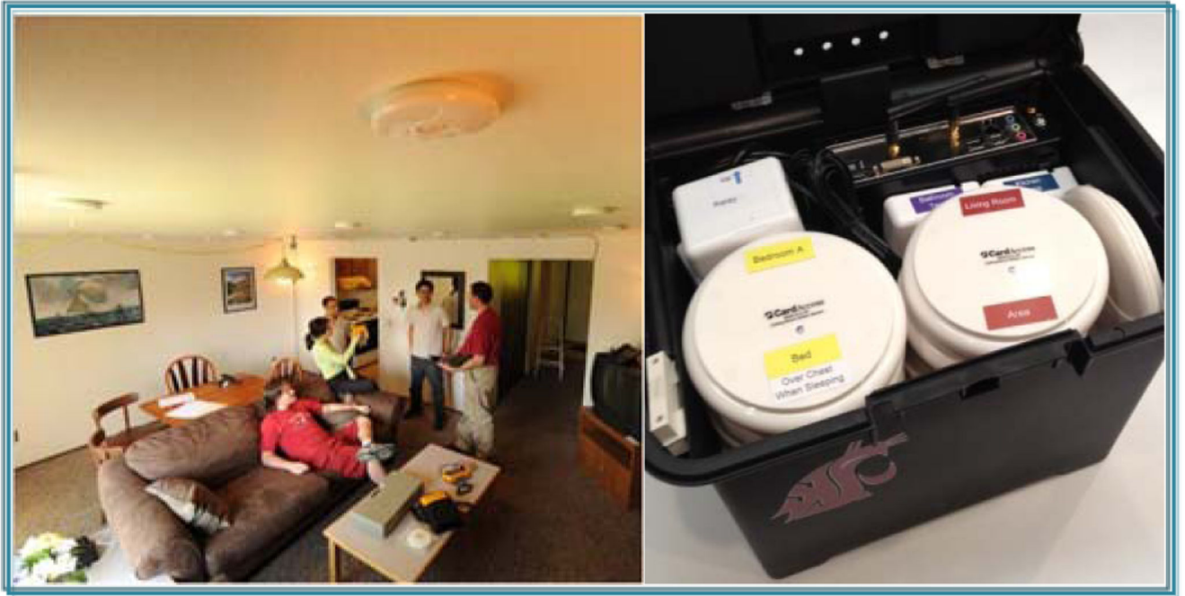
Figure 1. (left) Motion/light sensors and door/temperature sensors are installed in a smart home; (right) the SHiB kit includes sensors, computer, and networking equipment.
