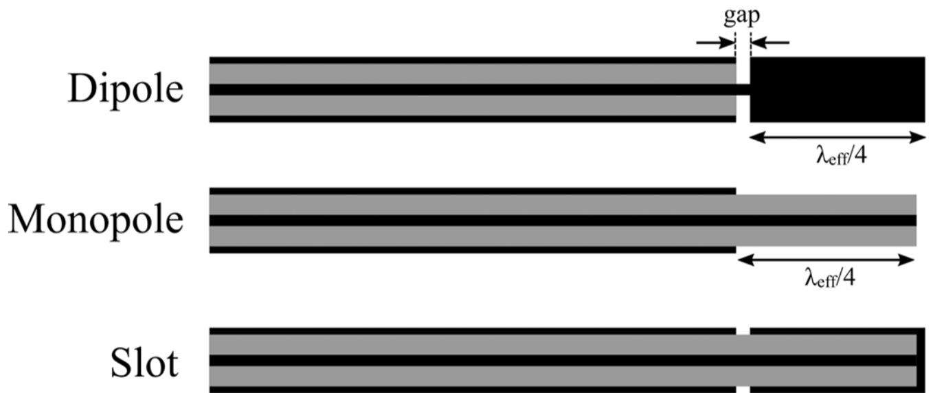
FIG. 6: Early MW antennas for interstitial thermal therapy: dipole, monopole, and slot (black: metal, grey: dielectric)
