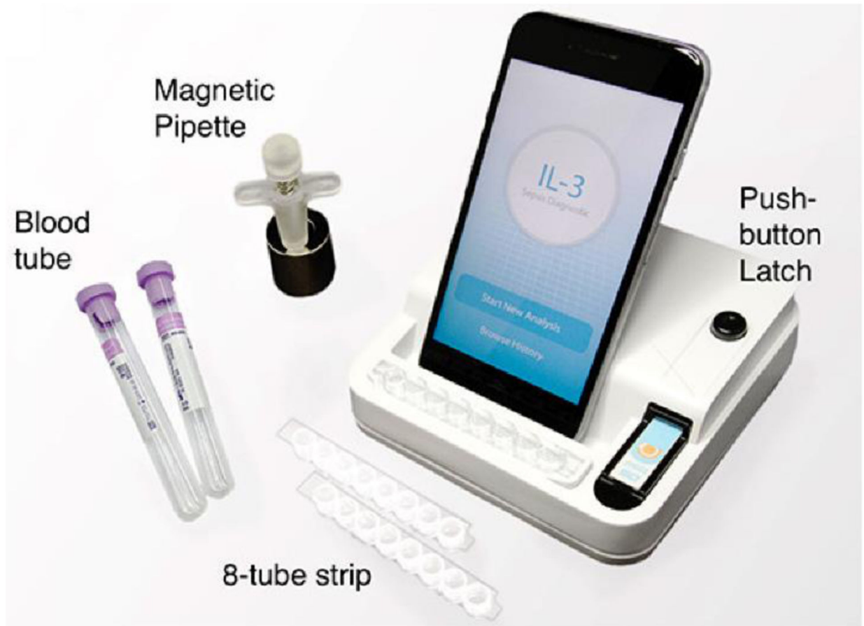
Figure 2. Example smart phone enabled POC interleukin detection device. Reproduced with permission from Ref. 53.
