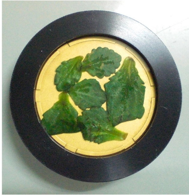
Figure 8. Sample cell for spectral measurement. All leaves of Haberlea rhodopensis were set in this case.
