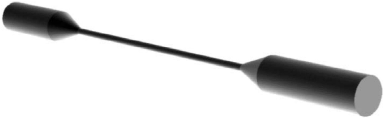
Figure 2. Solid model of capillary tube for CFD analysis. The test segment is 1 mm diameter and 70 mm length and is fitted at each end with conically shaped connectors 8 mm length.).
