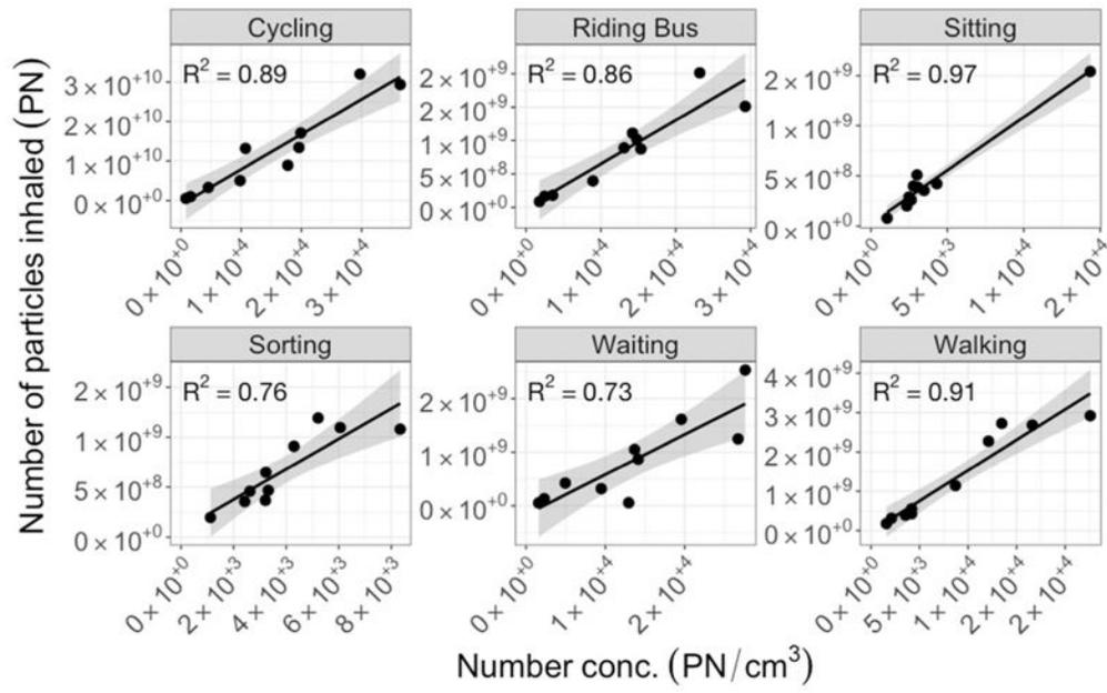
**Figure 4.** Number concentration versus number of particles inhaled by task, with linear regression (black line) and 95% confidence interval (grey shading).
