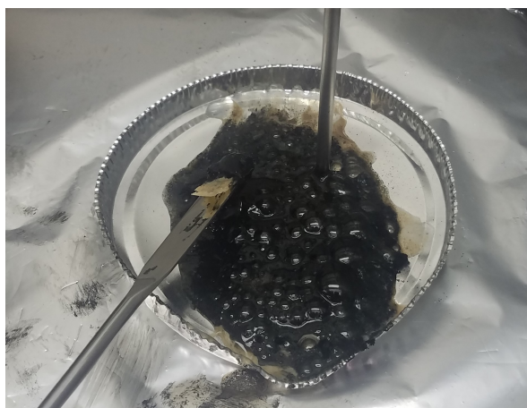
Figure A1. Reaction of 80:20 PHBV:PLA with BioC. Reaction occurs in close proximity to the melting temperature.
