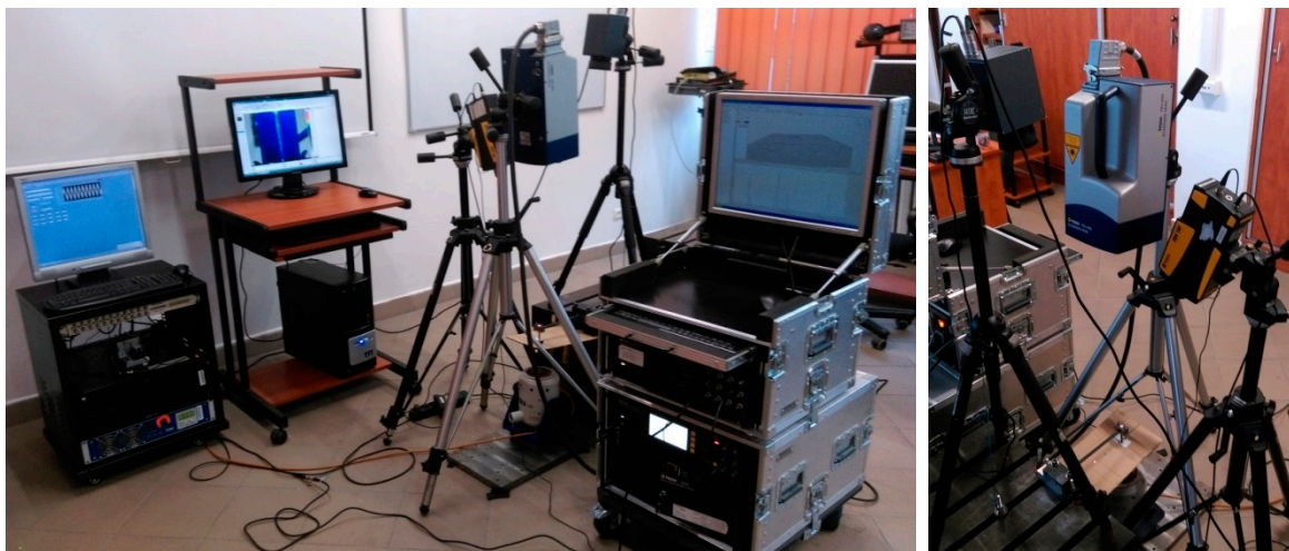
Figure 21. Testing apparatus for performing self-heating-based vibrothermography (SHVT) tests.
