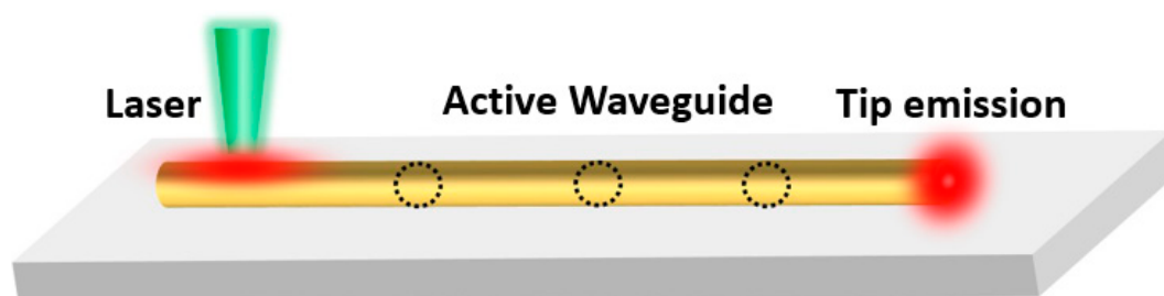
Figure 7. Scheme of waveguide loss coefficient measurement.
