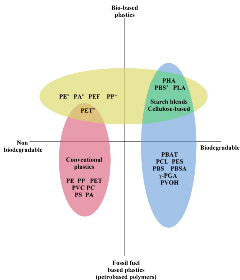
Figure 1. Plastics and bio-based polymers' diversity and comparison diagram. Abbreviations include: PA—Polyamide, PBAT—Polybutyrate Adipate Terephthalate, PCL—Polycaprolactone, PE—Polyethylene, PEF—Polyethylene Furanoate, PES—Polyether Sulphone, Polyethylene Terephthalate—PET, PP—Polypropylene, PC—Polycarbonate, PHA—Polyhydroxyalkanoate, \gamma -PGA—Poly(Gamma Glutamic Acid), PLA—Poly(Lactic Acid), PS—Polystyrene, PBS—Poly(Butylene Succinate), PBSA—Poly(Butylene Succinate Adipate), PVC—Polyvinyl chloride, PVOH—Poly(vinyl alcohol), adapted from [13]. The * indicates polymers that have bio-based origins plus fossil fuel synthesis routes.
