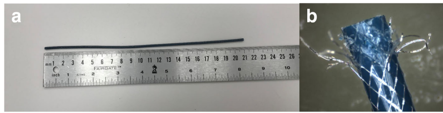
Fig. 5 a 21 cm long dissected segmented braided catheter subassembly part and b detached and scraped braiding wires
