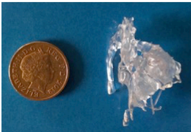
Figure 4. Foetal ultrasound images were used as input to create a 1:1 3D model of a foetal heart. Foetal heart models can be printed also in bigger scale to better appreciate small cardiac structures. In this image, a foetal heart model is compared to 1-penny coin (diameter 20.3 mm)
