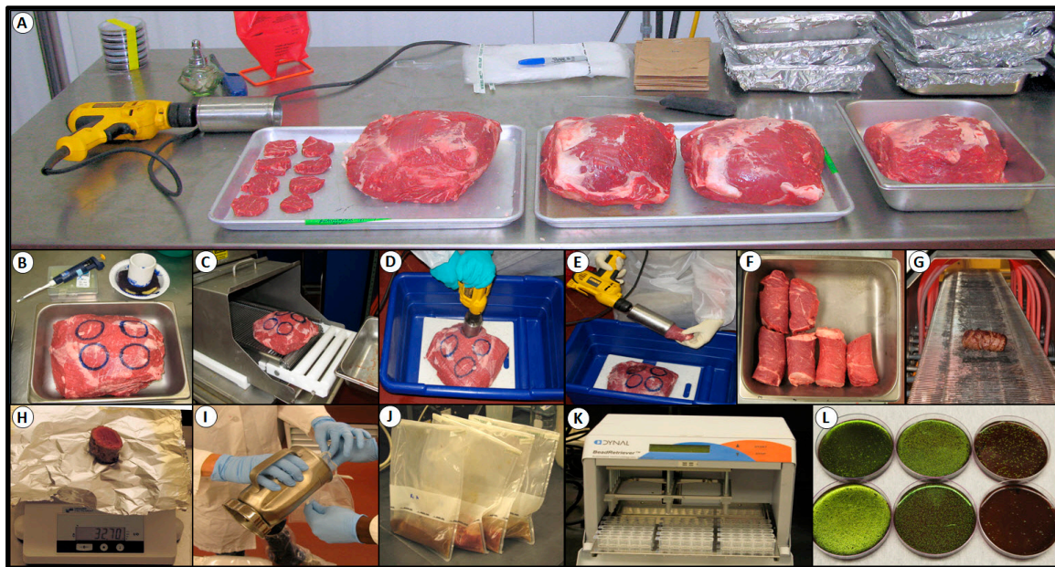
Figure 2. Phase 2, evaluation of select antimicrobials against E. coli O157:H7-inoculated beef subprimals in conjunction with blade tenderization. (a) Array of beef subprimals during one trial; (b) beef subprimal prepared for inoculation in labeled zones; (c) inoculated beef subprimal entering blade tenderizer; (d) sprayed and blade-tenderized subprimal being cored; (e) recovery of beef cores using a two-inch circular drill bit; (f) recovered beef cores; (g) sanitizing outside of beef cores by passage through radiant heat oven; (h) sectioning of beef cores; (i) blending and (j) enrichment incubation of beef sections; (k) Bead Retriever™ for immunomagnetic bead recovery and enrichment of E. coli O157:H7 from enrichment broth; (l) plating of immunomagnetic beads with recovered E. coli O157:H7 onto EMB media containing rifamycin SV.
