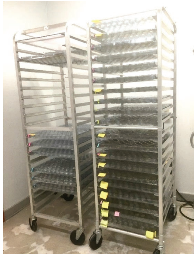
Fig. 6. Standard aluminum restaurant-style bun rack holding the custom cell trays.
