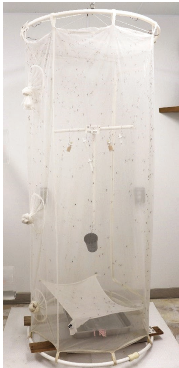
Fig. 2. The Tx. rutilus cage with hanging sugar feeders, water, and oviposition cup. In the bottom of the cage is the pupa emergence pan and screen cover.
