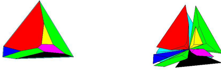
Fig. 7. Left: Laguerre cell that contains generator's center. Right: Pyramidal decomposition of Laguerre cell. All volumes are positive.
