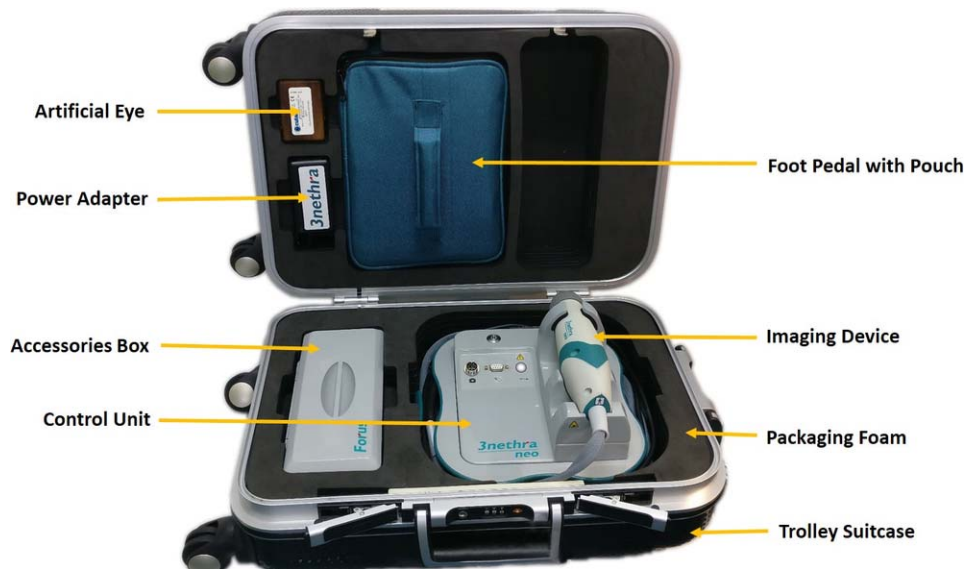
Figure 1. The Neo device with the cables, foot switch, and accessories placed in a single portable suitcase.
