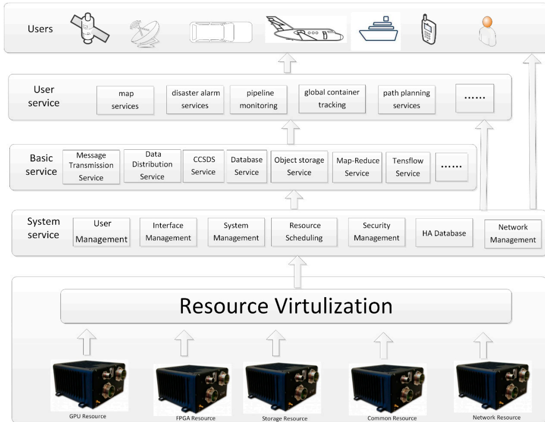
Figure 1. The framework of 5GsatEC.
