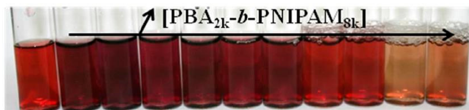
Figure 12. Image of the final NPs solutions 5 min after reduction at 20 °C. The polymer concentration increases from left to right (0 to 0.15 wt %). Reprinted with permission from [96]. Copyright 2010 American Chemical Society.
