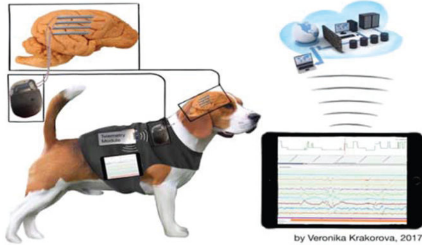
Figure 10: Illustration of brain coprocessor events from chronic brain recordings in-vivo: events are collected using the on-chip detection algorithms to trigger the detector when seizure-like activity is seen. [29, 32]
