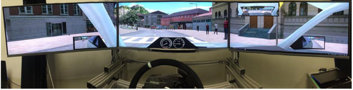
Figure 1: Scene from the driver's point of view through the virtual windshield, with rear view mirror, side view mirrors and a simple dashboard including speedometer and rpm as well as a pedestrian target on the far right of the center screen.
