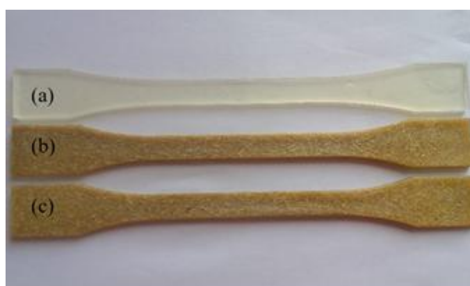
Figure 1. The shape of the composite materials. (a) PLA; (b) PLA/Wood; (c) PLA/Wood fiber/poly(lactic acid grafted with maleic anhydride (MAH-g-PLA)).
