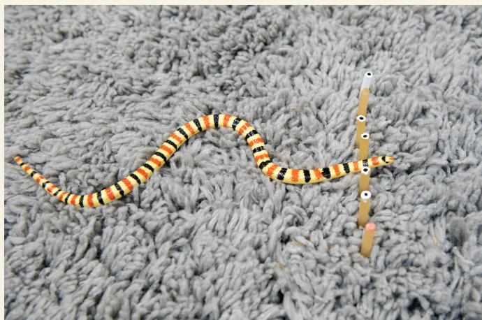
Shovel-nosed snake moves through force-sensitive rubber pegs. Image courtesy of Allison Carter (Georgia Institute of Technology, Atlanta).
