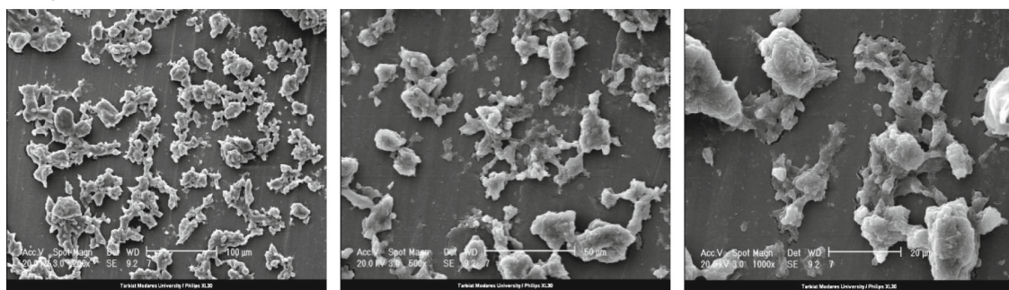
Fig. 2 Scanning electron micrographs of the different fucoidans (× 200; × 500; × 1000, left to right respectively)
