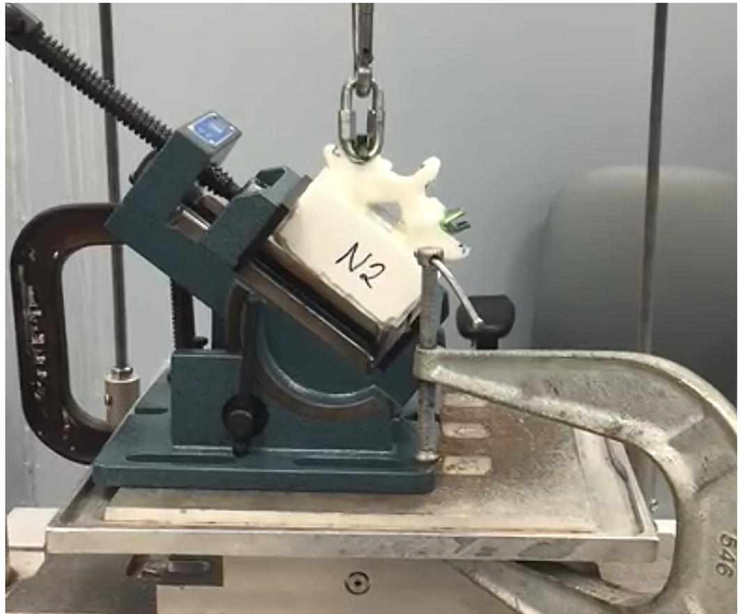
**FIGURE 3: Vertebral body model in the angled vise grip during axial pullout (APO) testing.**
