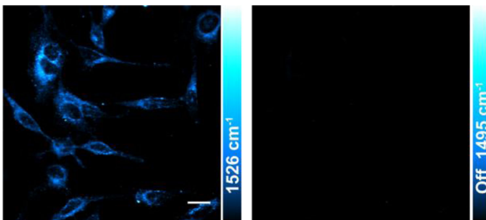
Figure 6. er-SRS imaging of IR820 in live HeLa cells with low laser power. Laser power used were P_{\text{pump}}=1 mW and P_{\text{Stokes}}=14 mW. Scale bar, 20 \mu\text{m} .
