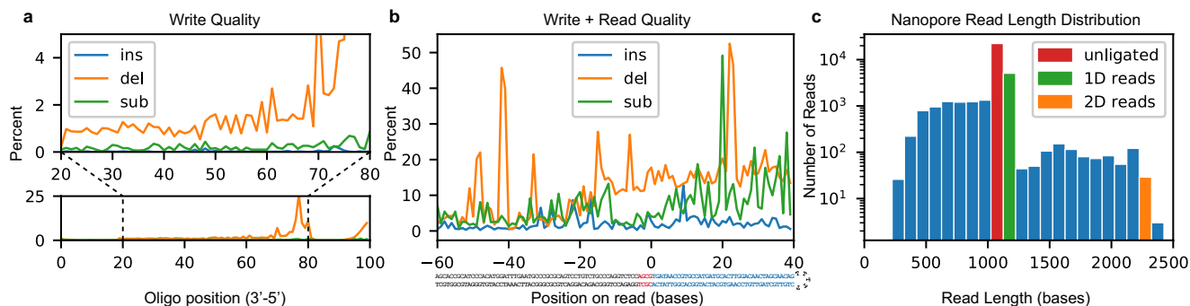
Figure 2. Synthesis and sequencing process quality. (a) Insertion, deletion, and substitution frequency by locus for a synthesized and PCR-amplified 100-mer. Below: An overview of errors. Above: An expanded view of the central 60 bases. The terminal 20 bases come from primers used in amplification and therefore are not representative of synthesis quality. (b) Combined write-to-read quality of synthesis, ligation, and sequencing. Bases -60 to -4 (below, grey) are adapter bases. Bases -3 to 0 (below, red) are the ligation scar. Bases 0 to 39 (below, blue) are the synthesized payload region with 8 bases of padding on the 3' end. (c) Distribution of nanopore read lengths with unligated, 1D and 2D read lengths identified.
