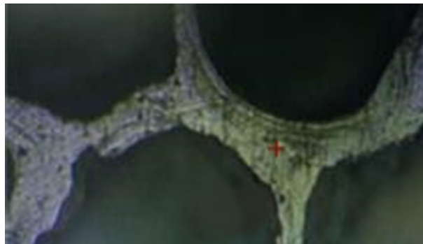
Fig. 2 Indentation sites for nanoindentation test. Actual indented sites were marked by red cross under optical microscopy, and the sample thickness was 2 mm
