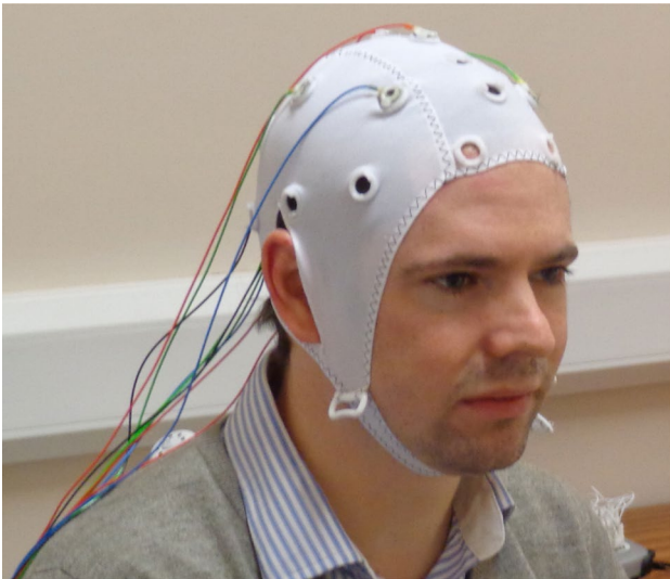
Fig. 1 A conventional lab based EEG set up with metal electrodes on the scalp held in place by a cap with wires to connect to a recording instrumentation box
