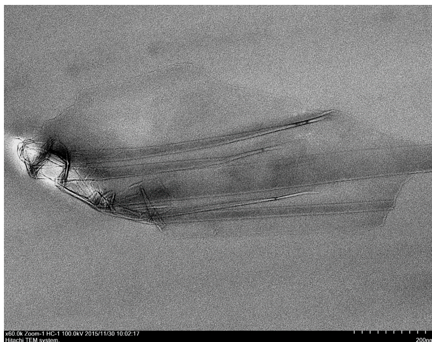
Figure 13. Cross section TEM image of RGO.
