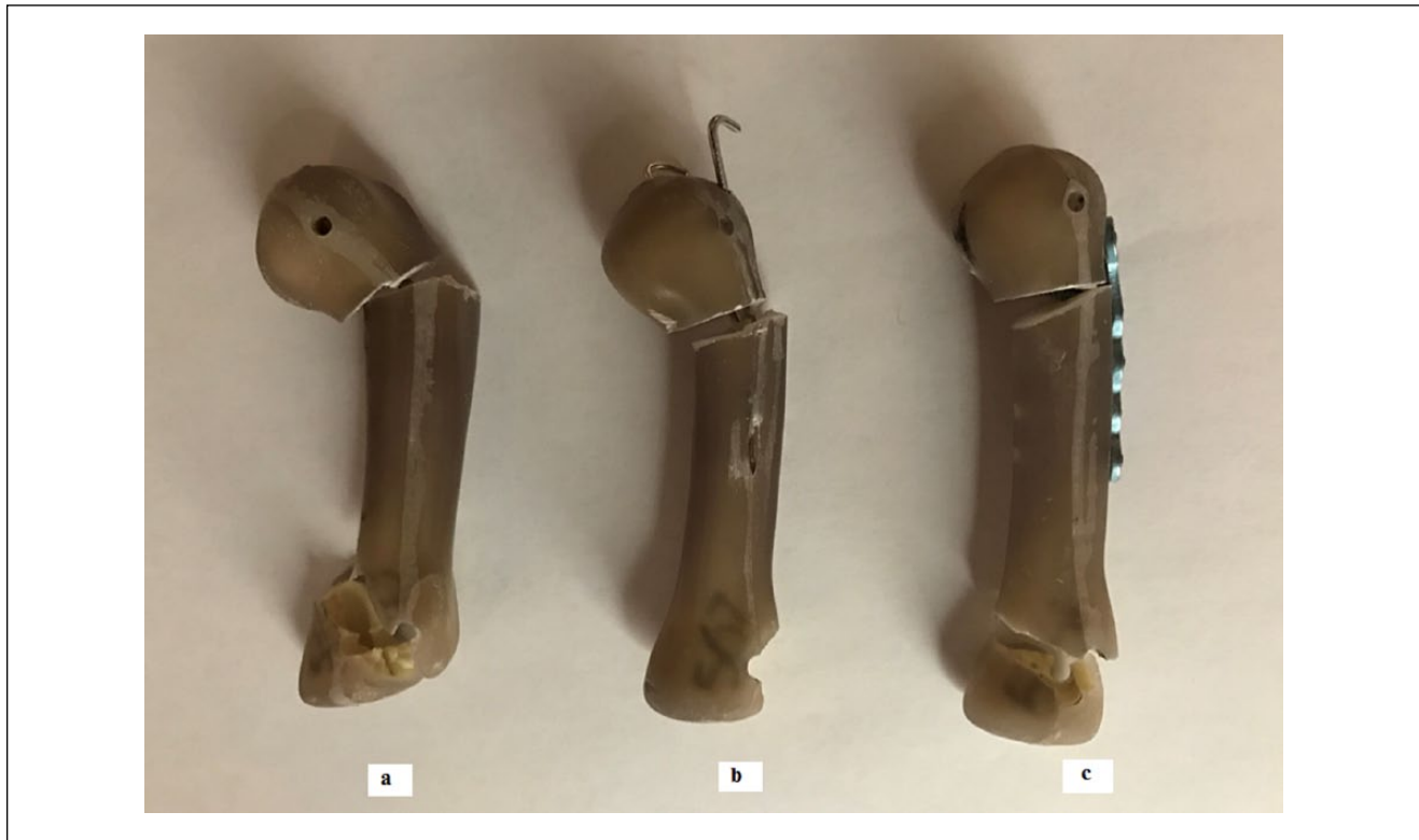
Figure 4. View of the models of the fracture fixation constructs after failure: 3.0-mm retrograde screw—HCS (a), 1.2-mm Kirschner wires—KW (b), and 2.0-mm dorsal T-plate with six 2.0-mm locking screws—LP (c).
