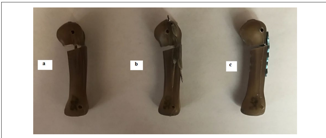
Figure 2. Representative models of the fracture fixation constructs: 3.0-mm retrograde screw—HCS (a), 1.2-mm Kirschner wires—KW (b), and 2.0-mm dorsal T-plate with six 2.0-mm locking screws—LP (c).
