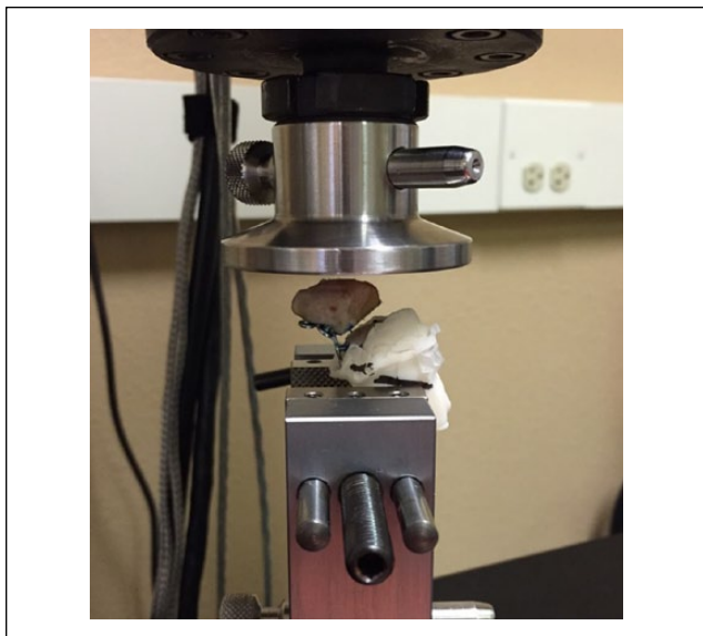
Figure 1. Scaphoid cadaver with plate fixation mounted on load frame.
