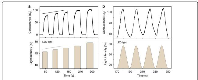
**Fig. 2 Conductance vs time as modified by the light intensity and light excitation form. a** Bottom panel: The incident light is periodically switched on and off, while the maximum light intensity in each circle is gradually increased. Top panel: the conductance of the metallic contact increased following the trend of the light intensity. **b** The conductance of the metallic contacts changes similarly to a sinusoidal wave, following the sinusoidal light intensity waveform
