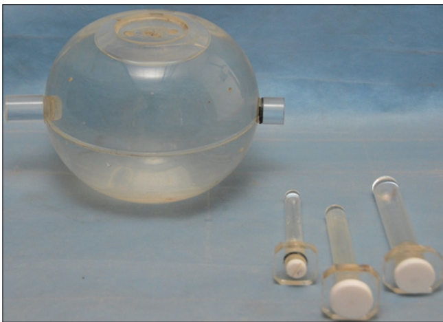
Figure 1: Calibration phantom consisted of two parts the outer sphere and the inner cylindrical tubes of various sizes to accommodate different size of pellets. The cylindrical tubes could be fitted to outer sphere with the help of a zig. The pellets of calibrators and validators were put in cylindrical tube which was inserted into outer sphere containing water. The inner cylindrical tube also contained a suitable liquid
