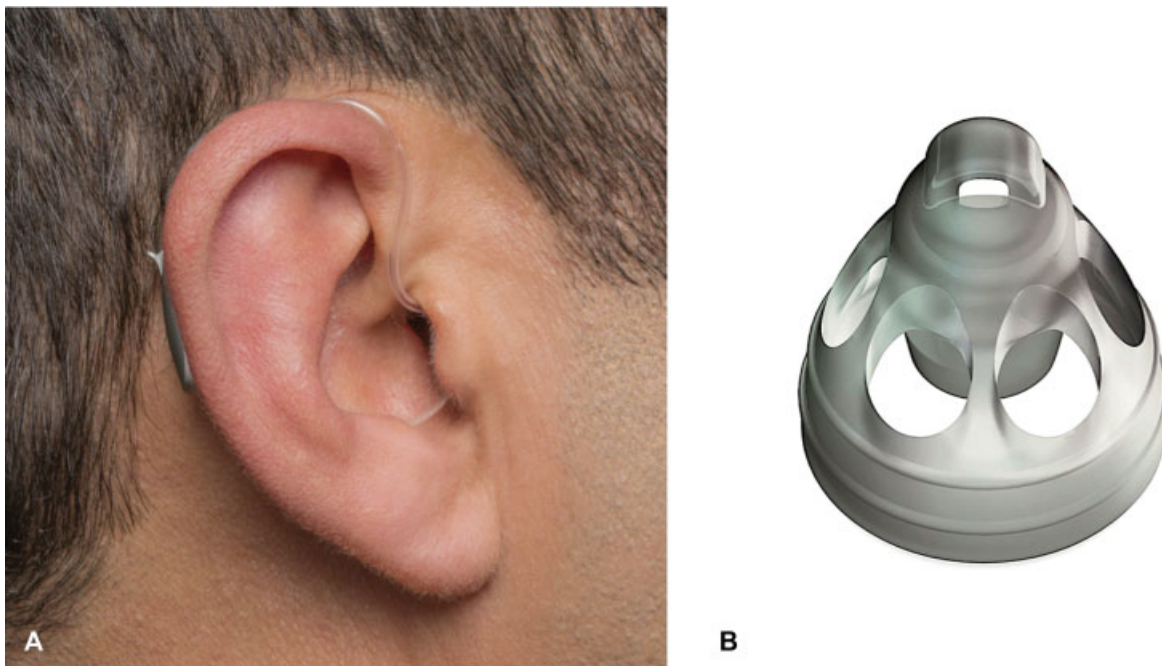
Fig. 2 The illustrations show current open fit CROS hearing aid configurations. Here, the hearing aid processor/transmitter is behind the pinna and the signal is delivered via a small thin tube (A) with an open dome (B) allowing for minimal obstruction of the natural ear canal acoustics (Images courtesy to Phonak, LLC, with permission). CROS, contralateral routing of signal.
