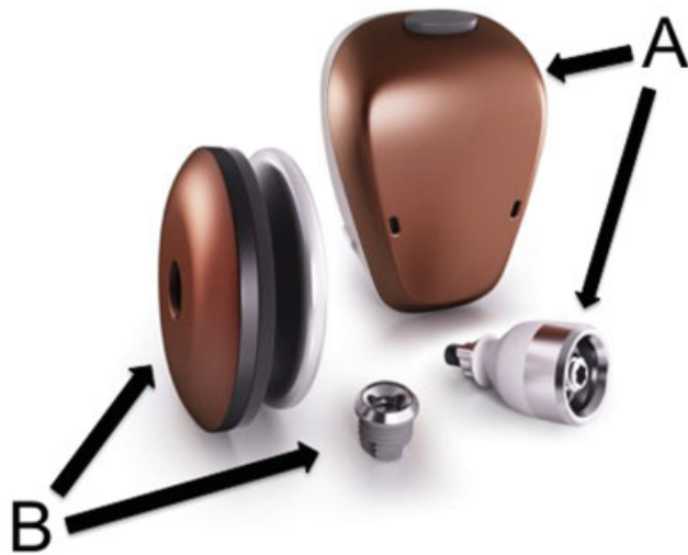
Fig. 6 (A) Cochlear Baha Connect (percutaneous) and (B) Baha Attract (transcutaneous) implants. Images provided courtesy of Cochlear Americas, 2014 Cochlear Americas.
