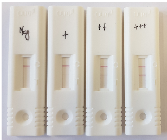
FIG 1 Lateral flow devices, showing from left to right a negative result, followed by increasing test line intensity. The control line is visible at the top, while the test line appears below the control line.
