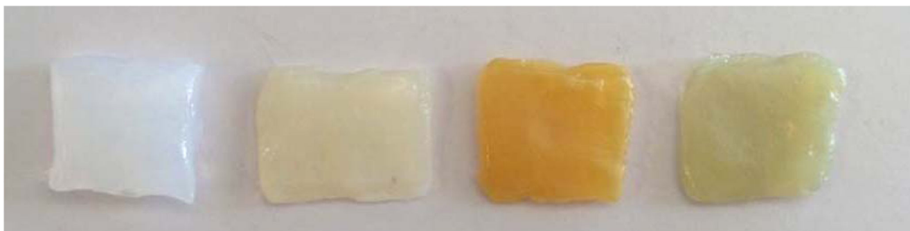
Figure 1. Macroscopic appearance of the wet BC membranes incorporating the different ILs. From right to left: BC, BC-[Chol][Caf], BC-[Chol] 2 [Etl], BC-[Chol][Gal]. The membranes produced had 62.12 \pm 4.40 % of water content.
