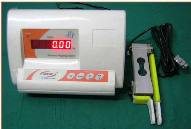
Fig. 3 Bite force device with digital indicator
