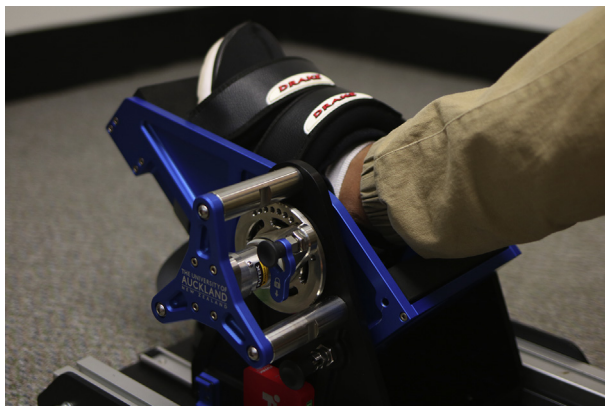
Fig. 2. Footplate measuring the torque around the ankle joint during isometric contractions.
