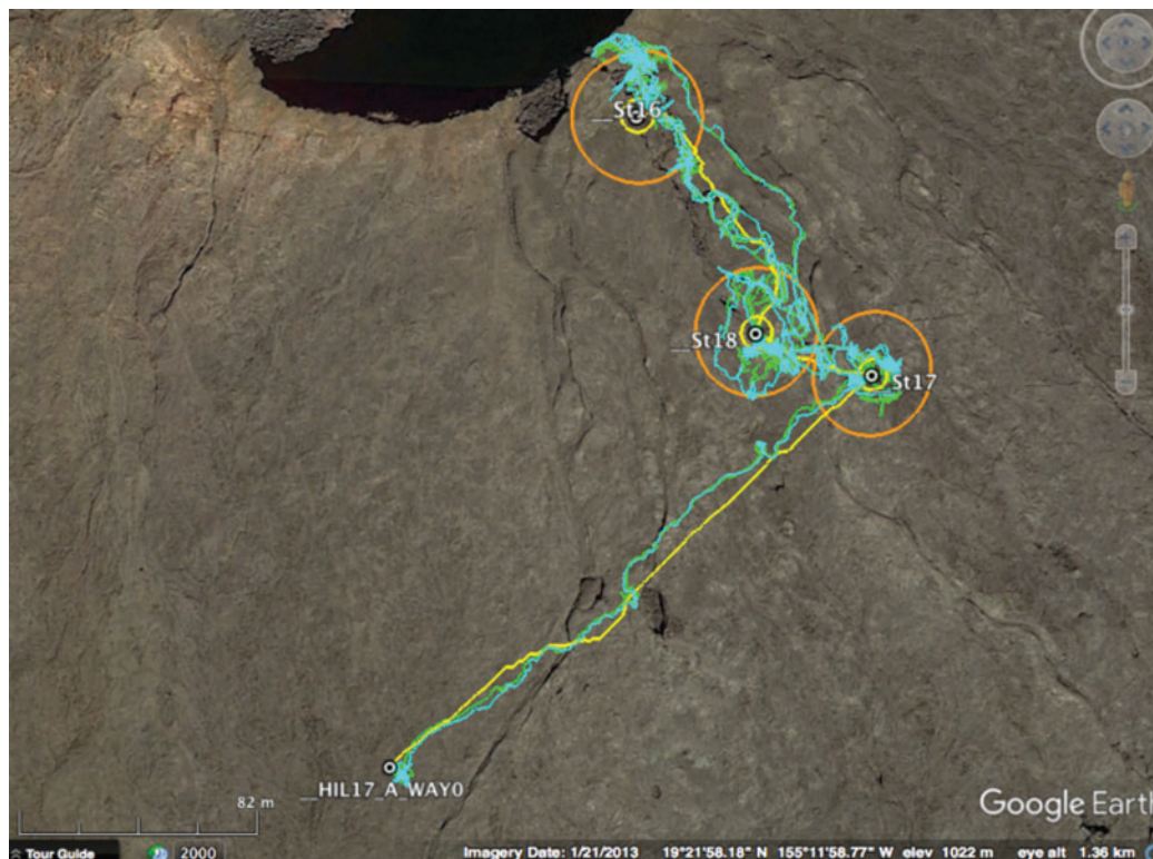
FIG. 3. Planned (yellow line) and actual (green and cyan lines for EV1 and EV2, respectively) traverses for EVA 7. Yellow circle = 10-m diameter station boundary; orange circle = 40-m diameter approach circle around station.
