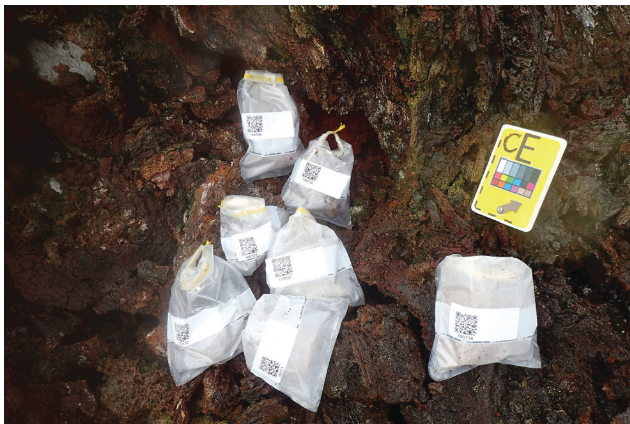
FIG. 10. A suite of samples collected from a “CE” candidate location. Each set of sampling ended with a similar photograph of sample bags in situ to provide context and specific localization.
