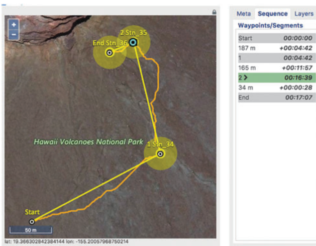
FIG. 7. xGDS showing stations (yellow circles), SEXTANT (curved orange lines between 2 stations), and SEXTANT timing (right panel).
