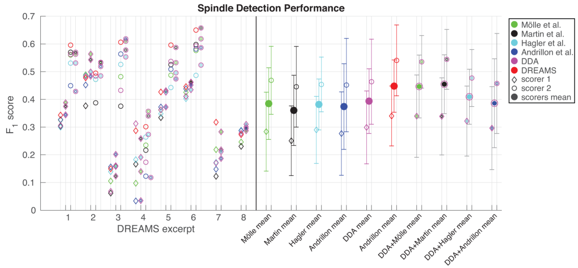
Figure 6: Spindle detection on DREAMS data. F_1 score is plotted for a set of automated spindle detection methods and DDA for the eight surface EEG excerpts included in the DREAMS data set. For six of the eight excerpts, two human experts scored the data. For these six recordings, F_1 scores based on the first expert’s markings are plotted as diamonds at left, and the scores based on the second expert’s markings are plotted as open circles at right. The means (diamonds and open circles) and standard deviations (bars) across all recordings for each detector’s agreement with both experts are plotted at the far right with the same markers, and the means of each method’s agreement with both scorers are plotted as larger filled circles. Combinations of the other measures with DDA, as shown in Fig. 5 are shown with the colors for each of the methods combined. In addition to the six methods shown previously, we also show here the F_1 scores of the automated spindle detections included with the DREAMS data with both human experts in red.
