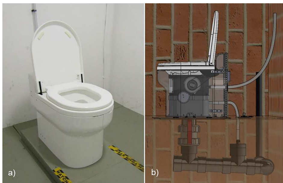
Fig. 2. a) Prototype pedestal with mechanical waterless flush, installed in a dedicated toilet room adjacent to the laboratories of the Pollution Research Group at the University of KwaZulu-Natal; b) schematic of the installation: The pedestal is connected to the sewer mains and has a ventilation pipe from inside the unit. The gear system is shown to be on the side of the pedestal, underneath the cover.
