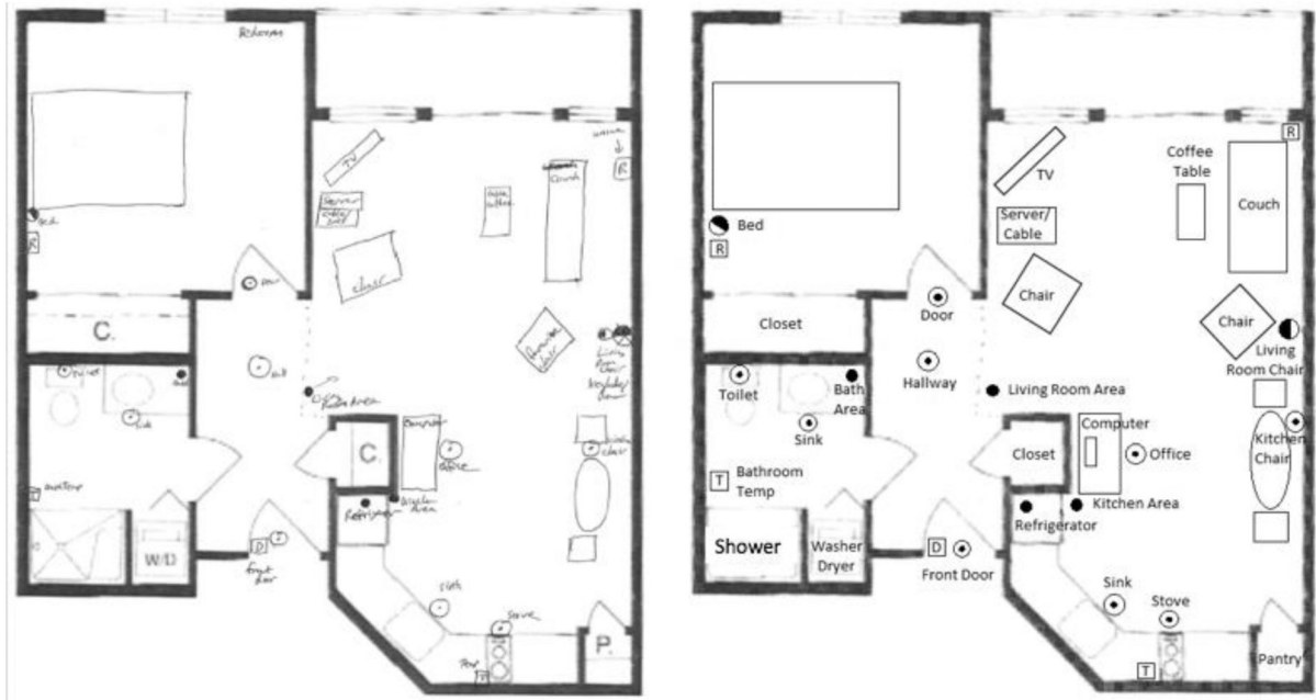
Figure 2. Floor plan of residence with field notes of furniture locations and the plan for sensor location by type ( Left ) and a digital copy that is created after the visit ( Right ). ○ direct sensor ceiling; ● direct sensor wall; ● area sensor; R relay; T temperature-humidity.
